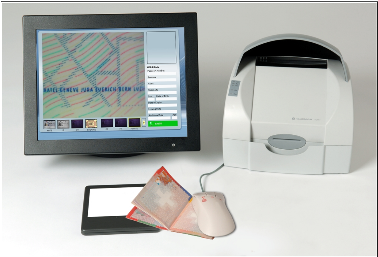
Reading of Microtext in reflection mode under different light sources, enlargement 30x
